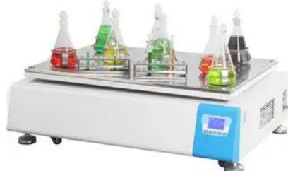
Microprocessor PID controller, with timing function, resume operation automatically if power off unexpectedly.
