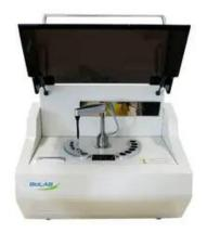
Optical Coagulation testing theory, PT derived FIB function. With automatic and manual dual mode test functions. Use tilt reagent position, avoid wasting, With LED lighting function. Sampling probe with liquid level sensor and constant heating function, avoid cross contamination
