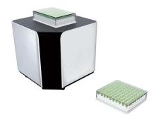
It can be finished within 5 seconds for one of 96 holes rack or 384 holes rack. Advanced decoder technology can be identified as stable and secure even if the code is fuzzy.
