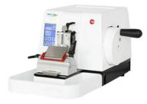
Full-automatic sectioning with adjustable speed and three sectioning modes continuous, step and single. LED display. Electronic trim function makes it easy to switch from trim and section mode. Specimen retraction mechanism protects specimen from unintended blade damage. Section counting function counts total section pieces and total thickness.
