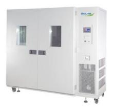
Microprocessor control, stainless steel chamber, semicircular arcs at corners for easy cleaning
