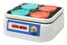
Microprocessor control with simultaneous display of time and speed Compact space-saving design fits easily in incubator and refrigerator Brushless DC motor ensures maintenance-free, reliable and quiet operation Adjustable speed control provides gentle to vigorous agitation Multi-functional shaking system Audio alarm signals program completion Accommodate a variety of platforms, non-slip rubber mat, conical flasks and other
