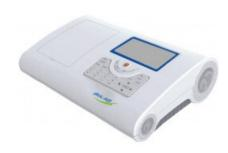
Double light path design can prevent circuit fluctuation and stray light to ensure stability of the instrument
