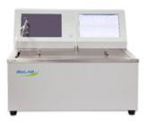
The instrument is used to make determination for vapor pressure of gasoline, volatile crude oil and other volatile petroleum products. It cannot be used to determine the vapor pressure of LGP. It is fully-automatic vapor pressure tester by PC control and operation. Advanced heating technology do separation of water and electricity meanwhile lower the height of water in bath. No blind angle in bath. It can save water and energy and also convenient to be cleaned.
