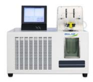
The instrument can be used to test freezing point of engine coolants and condensation liquids. Automatically judge the freezing point temperature. According to the different configuration, it can be used to test the freezing point etc.indexes of jet fuel, engine coolant and its concentrated solution, it's a multipurpose freezing point tester. It's the floor stand structure, the work table-board is made of stainless steel, concise design, nice appearance, convenient usage, fully furnished.
