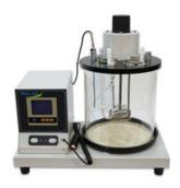
The instrument is suitable to determine kinematic viscosity of liquid petroleum products (Newtonian fluids )at a constant temperature. This instrument adopts hard glass bath and electric stirring device. Easy to observe the sample. The temperature in water bath is uniform.
