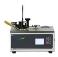
Single chip microcomputer control technique.LCD screen displays. The heating power is continuously step-less adjustable. The rate of heating up is exact.Easy setting for parameters. Press the "record"button when the flash point appears. The screen will show and reserve the flash point.
