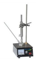
Comply with test requirements of antifreeze and brake fluid. Digitally display control voltage. High temperaeture resistant glass partition
