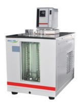
Low noise magnetic pump cross circulation structure. Can test density of antifreeze
