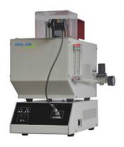
Automatic nonlinear curve temperature control, can be edited and drew in real-time according to requirements. Calculate and print borderline pumping temperature of Gas barrier type and flow limited type; Equipped with newly developed defrost system.
