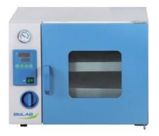
304 stainless steel, mirror polishing processing, easy to clean and maintain PID controller with over temperature alarm and timing function ensures precise and reliable control, also save more than 40% heating time A big dual layer tempered glass on the door provides good observation Door adjustment system with silicon door gasket ensures better vacuity
