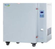
304 stainless steel, mirror polishing processing, semicircular arcs at corners easy to clean and maintain. The space between the shelves in the chamber is adjustable
