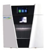
Comprehensive safety guarantee, combined with anti-corrosion capability Dual magnetron inverter control system ensures consistent sample digestion Two LCD screen, displaying real-time operation and experiment status Full-vessel precise temperature control and monitoring, ensuring safety and digestion performance.
