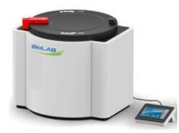
Special Designed Sample Digestion Vessel. Contact-less Temperature and Pressure Monitoring System. With vessel quantity of 40, It can edit and store 255 types of programs according to user's requirements.
