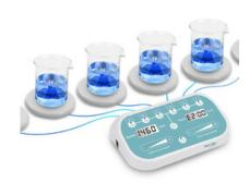
The BMMS waterproof stirrer can be put into a water bath or work in a high-humidity constant temperature box.
