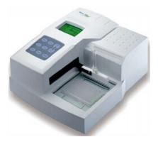
Easy Windows operation system, large LCD display. Washes flat, U and V-bottom strips and plates. 12-way or 8-way manifold, automatic and manual positioning. Large memory up to 50 wash protocols can be programmed. Automatic monitoring for vacuum and pressure, automatic rinse cycle. Washing pressure volume and time adjustable. Liquid level detection and alert function. No special airtight bottle required for wash bottle. Easy maintenance.
