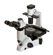
Excellent optical function with trinocular viewing head inclined at 45°. Innovative stand structure and sharp image display. Convenient operation and special design for viewing incubating cell tissue. Valid mould proof design. It can be used under the high temperature and high humidity environment.
