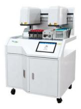
Safety: Automated Sample Processing System is equipped with high-efficiency filter and built-in UV lamp, and it can be used with a biological safety cabinet, to effectively prevent aerosol pollution
