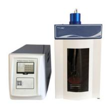
7 inch large screen LCD touch screen display. Microcomputer control, which can store 20 sets of work data. Ultrasonic time, ultrasonic power can be set.
