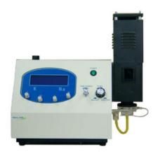
It meets the requirements of medical clinical test in addition to new added functions of testing high contected K and Na it has the detection function of Li salt taken by the mental patients.
