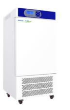
Balance Refrigeration Adopt without fluorine R134a refrigrant technology Duct circulation Stainless steel inner Programmable intelligent PID control Usd large capacity humidifier Double door design Lighting device With UV lamp
