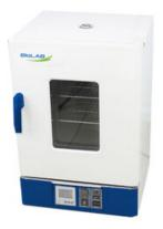
Micro-computer digital or liquid crystal temperature controller with LED digital display Stainless steel interior and cold rolling steel with electrostatic spraying exterior Door with double glass observation window and adjustable air-tight lock
