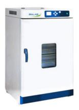
Stainless steel inner chamber with semicircular transition and adjustable shelves Easy to use interface
