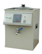
The full automatic procedure control&new heating element gives feature of quick heating & energy saving. It possesses the function of memorization to keep the set temperature automatically after startup. The LED shows heating state.
