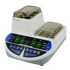
Unique dual temperature control slot can individually control temperature to make sure noninterference. One equipment to meet the demand for more experiments.
