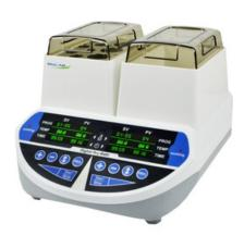
Unique dual temperature control slot can individually control temperature to make sure noninterference. One equipment to meet the demand for more experiments.
