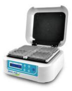
LCD display. Setting temperature and actual temperature simultaneously displayed. Diminishing time displayed.
