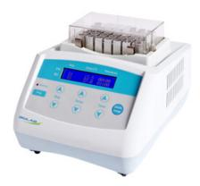
Microprocessor controlled incubation temperature and time
