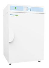
Microprocessor temperature and CO2 controller Water reservior volume: 3L Alarms: Power interruption, High/Low temperature, CO2 deviation, low RH programmable alarm, Door ajar, Independent over heat protection RS232 interface Type 304 Stainless steel shelves
