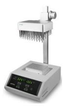
The heater heats the sample rapidly to the evaporation temperature, and at the same time, the gas is blown to the surface of the solution through the gas needle, which promotes rapid evaporation of the solution and concentration of the sample
