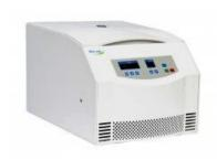
Brushless DC motor which is in great torque, free maintenance, no powder pollution, quick in speed up and down.
