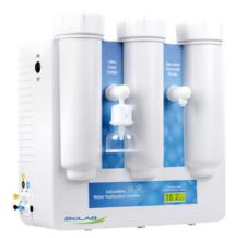
With tap water inlet, to produce RO water and ultrapure water, quality can reach to 18.2 M $\Omega$ .cm.
