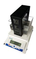
Density frame Electronic Balance RS232 interface
