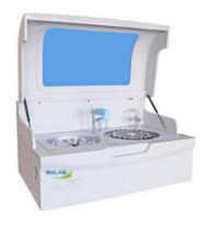
49 Sample positions.56 Reagent positions.120 Reaction cuvettes.200 Tests per hour.Probe with anti-collision function, liquid level detection function.
