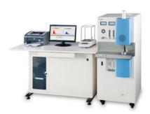
It can fleetly and exactly measure the carbon and sulfur in steel, iron, alloy, nonferrous metals, and other materials.
