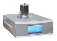
The main control chip of the instrument adopts Cortex-M3 core ARM controller, which has faster operation speed and more accurate temperature control. USB two-way communication makes the operation more convenient. Adopt 7 inch 24bit color LCD touch screen, the interface is more friendly. Adopt Ni Cr alloy sensor, more resistant to high temperature, corrosion and oxidation.
